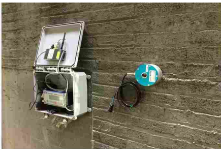
Figure 3. Installation of seismograph (at right) and monitoring data logger (at left) in progress at foundation wall of existing building.
