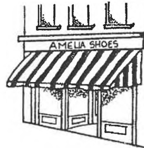
Sign on Exposed Lintel Or Clerestory
