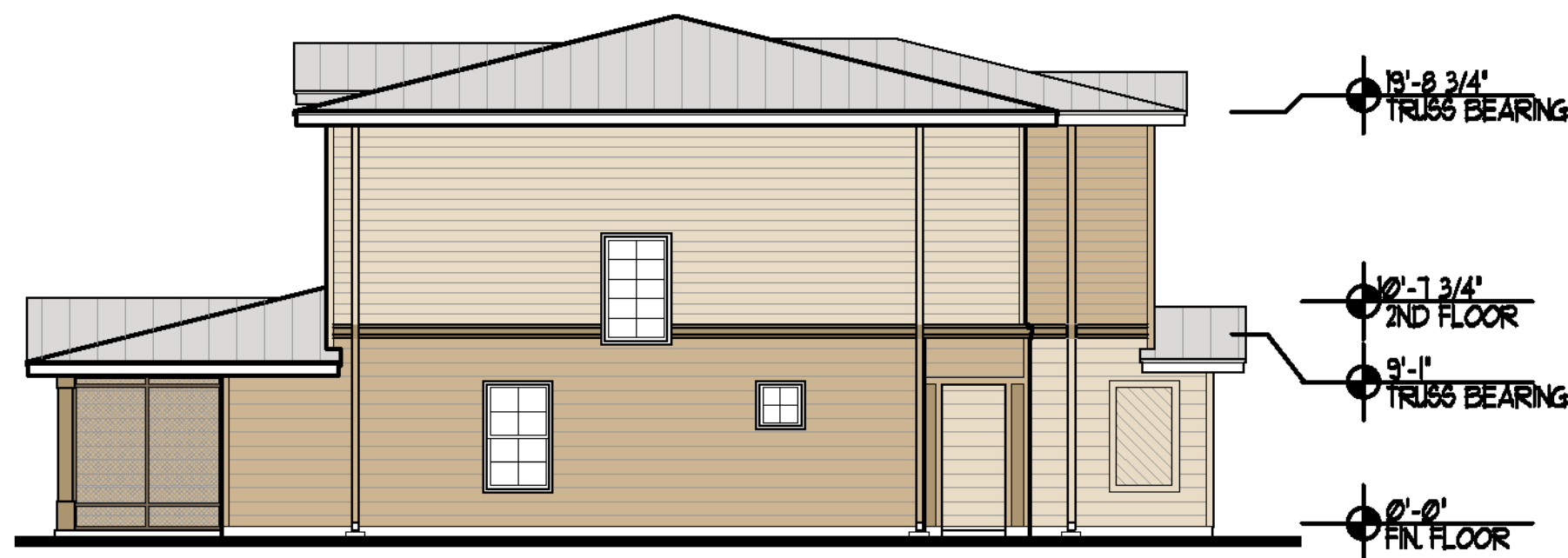
4 TYPICAL WEST ELEVATION (LEFT SIDE) SCALE: 1/8" = 1'-0"
