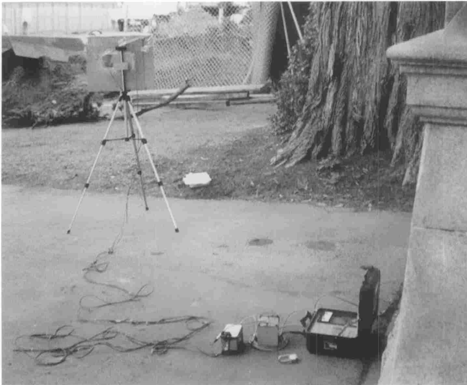
Figure 6. A seismograph records vibrations transmitted at the ground level of an historic building. The instrument is wired to a light and siren designed to warn the excavation crew that vibration levels are approaching preset limits. Additional sensors are often installed in the basement and on sensitive features such as stained glass windows. Photo: Wilson, Ihrig & Associates, Inc.
