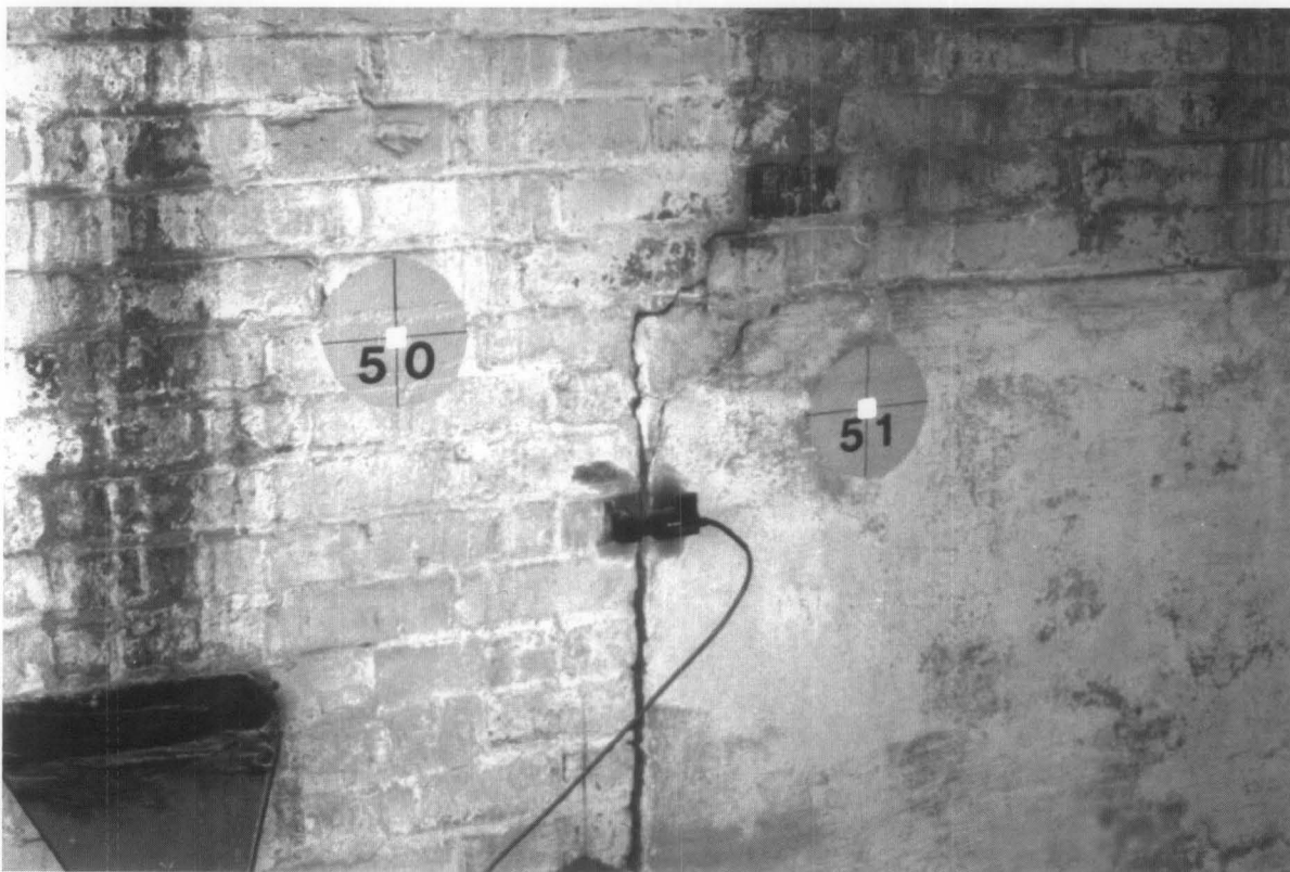
Figure 7. Electronic crack monitor and survey targets are shown installed on an existing wall. The crack monitor feeds movement data to a laptop computer. The targets are aligned and measured with optical survey equipment to determine the degree and direction of movement. Photo: McMullan and Associates, Inc.
