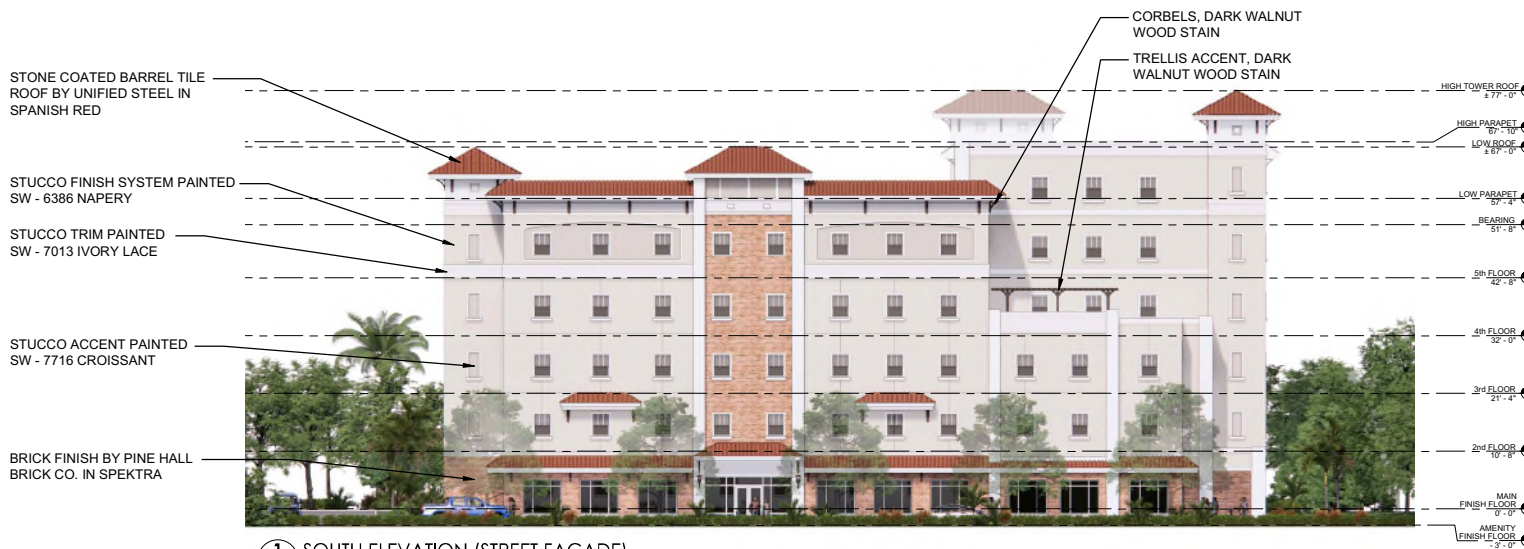
1 SOUTH ELEVATION (STREET FACADE) E-01 SCALE: 3/32" = 1'-0"
