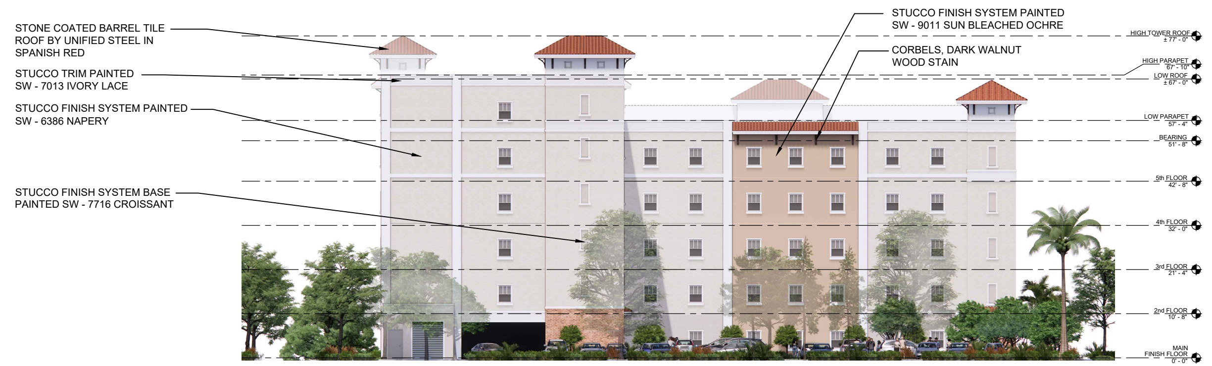
1 NORTH ELEVATION (REAR FACADE) E-02 SCALE: 3/32" = 1'-0"
