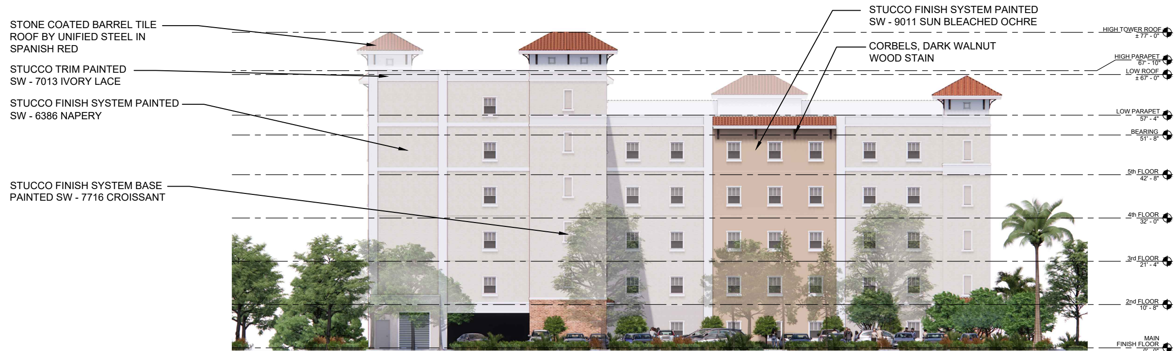
1 NORTH ELEVATION (REAR FACADE) E-02 SCALE: 3/32" = 1'-0"
